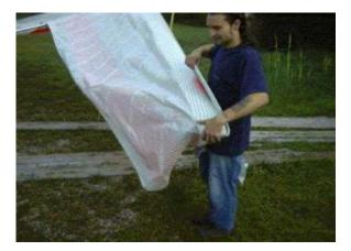
• Holding the extremity of the wing in this position, take the sail by the trailing edge and lift it upwards until it is tight and from this position roll in the sail, starting from the trailing edge.
