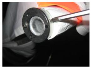
• Using a pair of needle-nose pliers pushed into the two holes in the head of the cam, rotate the cam to the degree desired. In the example described above, the cam will have to be rotated 5 mm anticlockwise.
