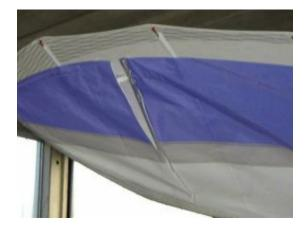
Make sure that the tip wire is free and running parallel to the tip; it must not be twisted around it! In
